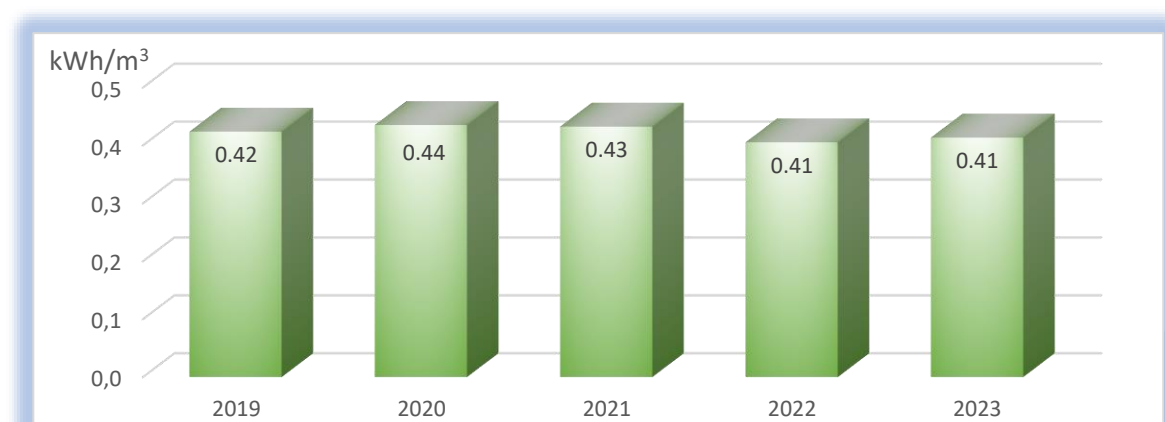
Chart 8: ELECTRICITY CONSUMPTION PER UNIT OF WATER PRODUCED AT THE WATER TREATMENT PLANT IN 2019–2023, kWh/m 3
