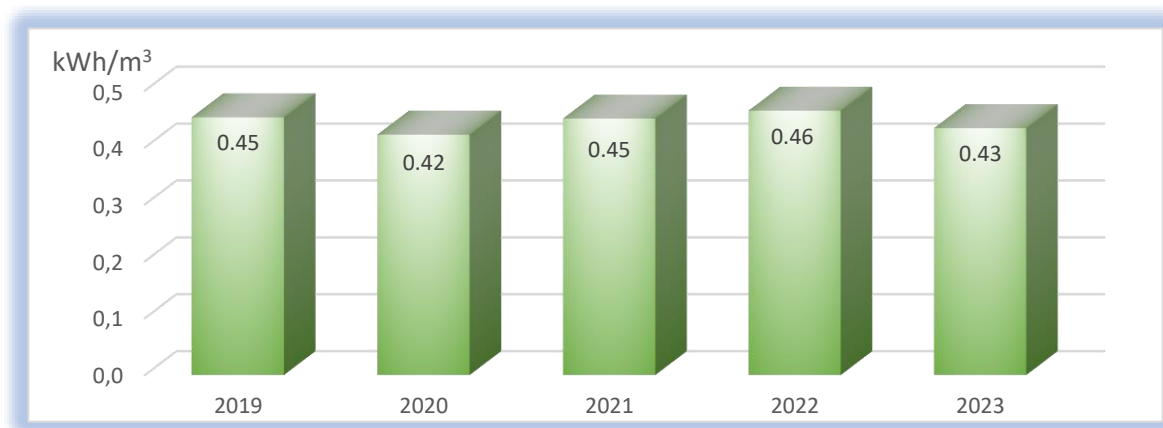
Chart 9: ELECTRICITY CONSUMPTION PER UNIT OF WATER PRODUCED AT THE WASTEWATER TREATMENT PLANT IN 2019–2023, kWh/m 3
