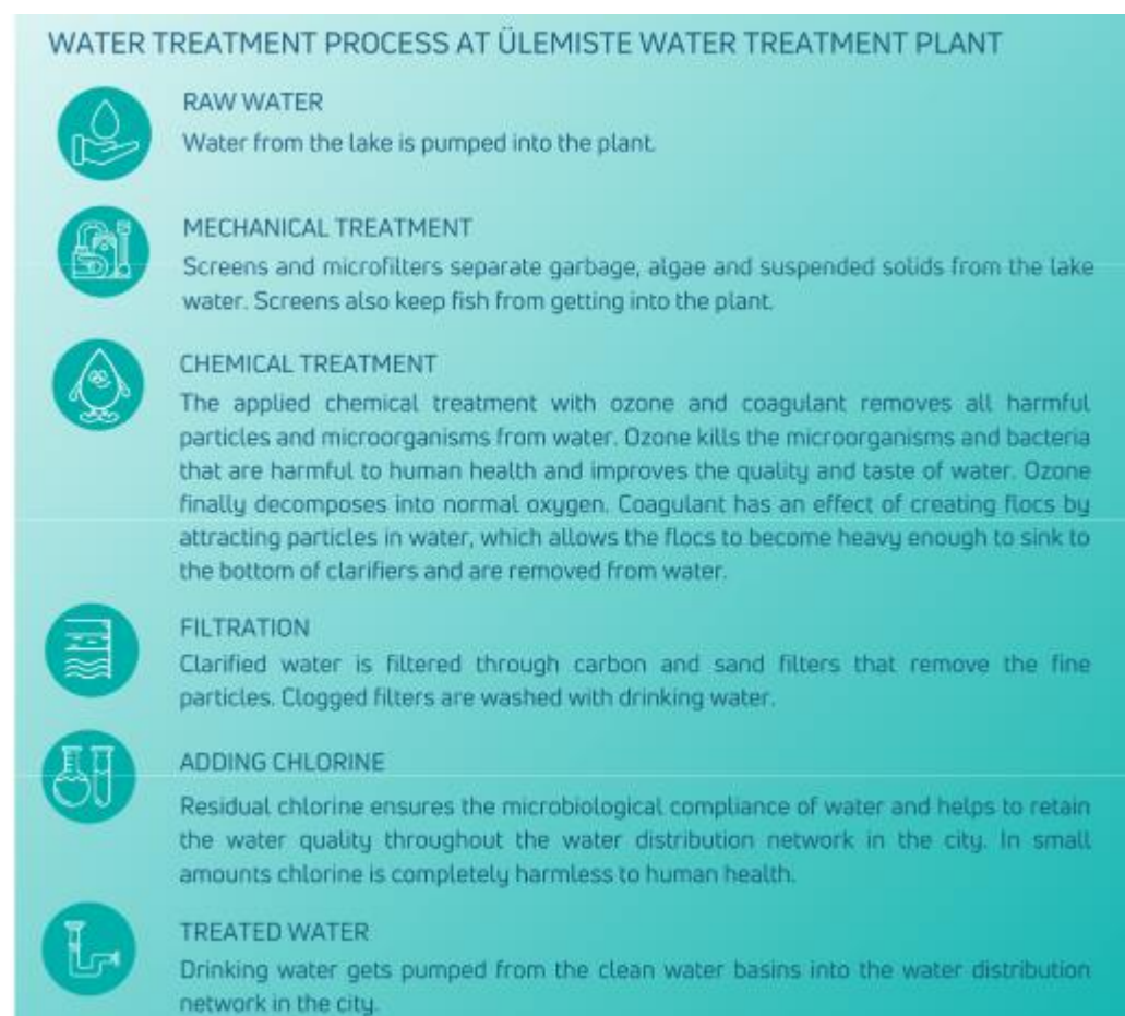
Figure 1: Water treatment process at Ülemiste water treatment plant
